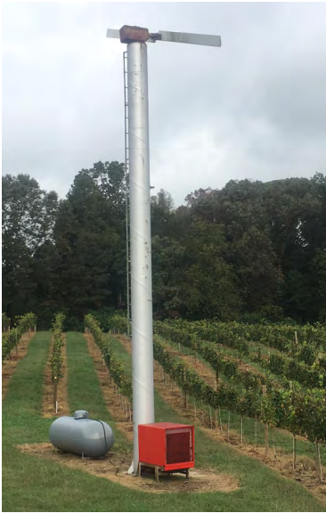
Figure 5. A wind machine in a young 'Chardonnay' vineyard during the postharvest period.
